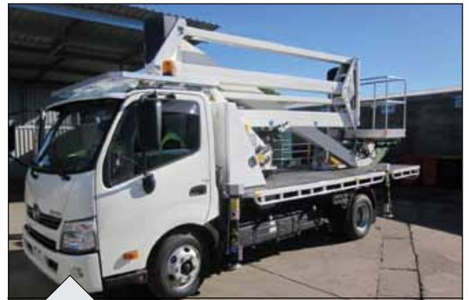
All hoses and wiring are neatly routed inside the PX boom sections, eliminating component damage in harsh applications such as tree maintenance works. The controls are simple, well proven, live hydraulic levers, which provide smooth proportional operation of the booms. A number of operations can be made simultaneously, increasing the speed and accuracy of movement even at full extension.
