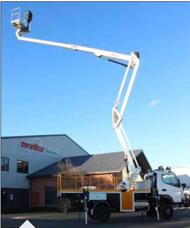
Not only do the PX models excel in horizontal reach, but they also provide a much better vertical lift path which is ideal for working up the face of buildings, signs etc. (209PX pictured on 4x4 Canter.)
