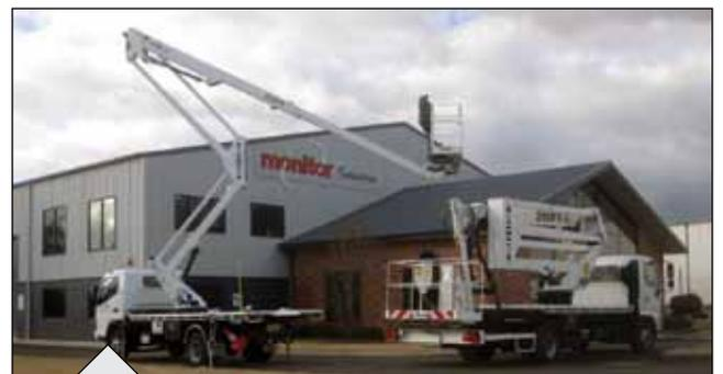
With a choice of stabilizer configurations and S.W.L. options, the PX range can be mounted to very compact and light weight commercial vehicles. In fact, we can even provide a 20 metre boom lift on a car licence!
