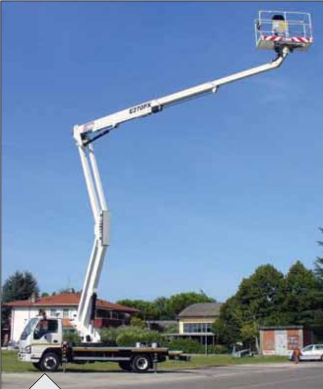
For superior up-and-over outreach, the "PX" design is choice number one! The modern double knuckle technology also provides a very compact machine without the problems of "tail swing" associated with conventional single-knuckle boomlifts.
