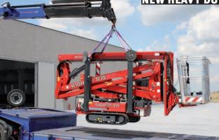
For handling by crane, once closed, the machine can be moved using ropes fixed on these new and practical hooks for cranes positioned at the end of the outriggers.
