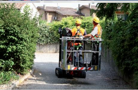
The innovative Auto2Speed traction system allows the machine to reach an optimal translation speed of 3.6km/h, to move quickly from one place to another on the construction site. Furthermore, thanks to the inclination control, the machine automatically decelerates in extreme conditions to enhance operator's safety.
