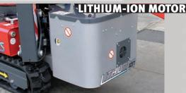
AVAILABILITY OF THREE ENGINES Honda petrol engine iGX440 + auxiliary 230V motor Hatz diesel engine with new "HD Autorev" technology for automatic acceleration and deceleration depending on the movements + auxiliary 230V motor Lithium Battery Pack 48 V - 90 Ah
